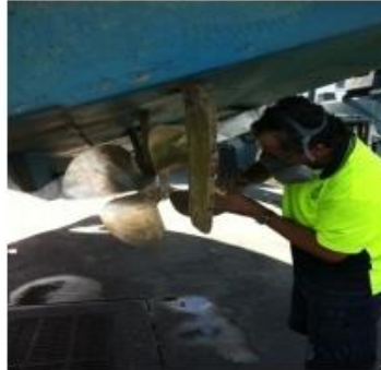
Surface preparation with grinder
